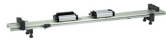
Figure 4.2 Low-friction track and carts used in the experiments described in this chapter.
